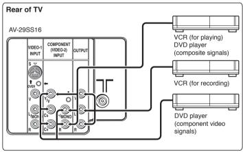
When connecting to COMPONENT (VIDEO-2) input, depending on the connection, choose the appropriate video input using the menu (see "VIDEO-2 SETTING" on page 16)
